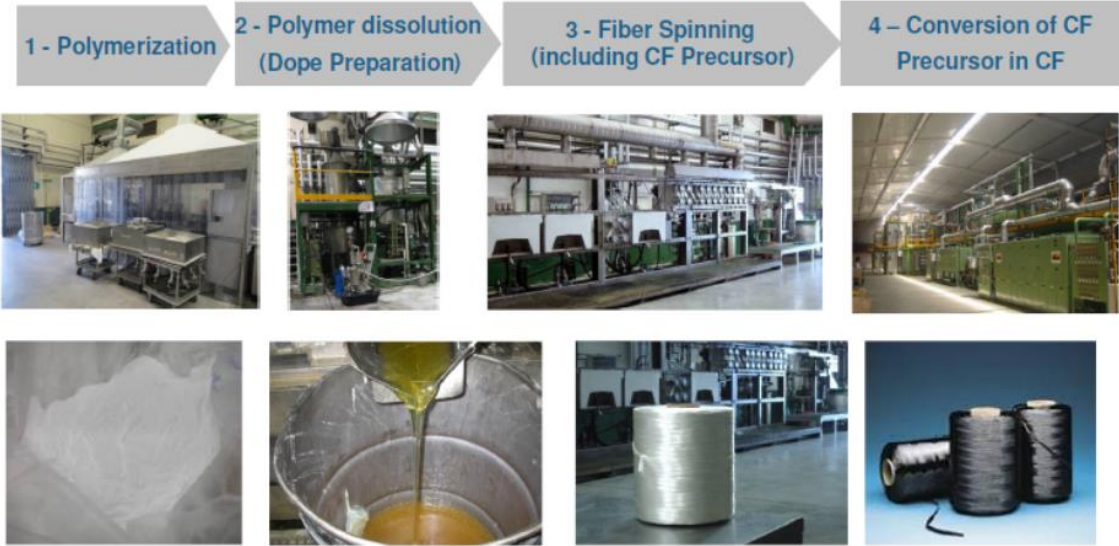
Figure 7 – FISIFE's manufacturing process of carbon fibers from PAN-based precursor [21].
