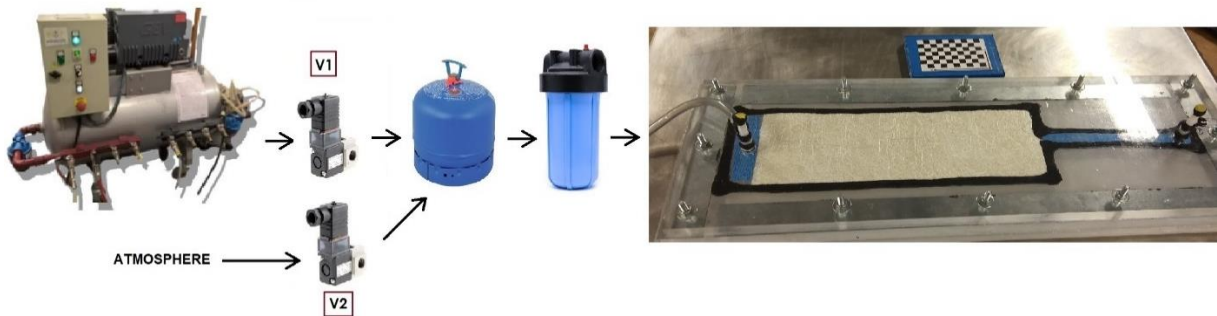
Figure 4 - schematic representation of the pressure control subsystem [5]
