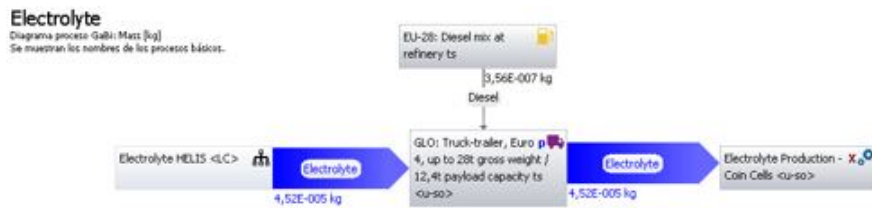
Figure B.5: The GaBi process flow is displayed for the electrolyte of the IREC battery. It only consists of transport since it is the same electrolyte used as in the HELIS battery.
