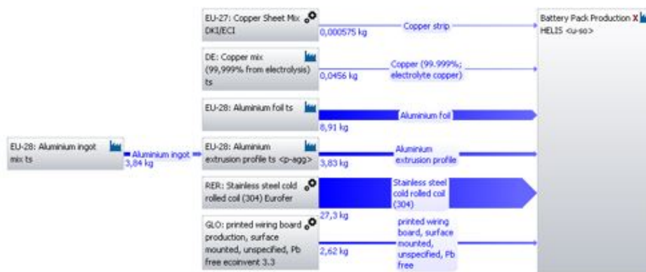
Figure A.6: The GaBi process flow is displayed for the battery pack (the same materials were used for the two battery systems).
