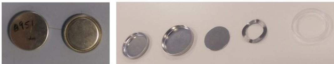
Figure 2.3: Photos of the cells manufactured by IREC (left) and their parts (right).
