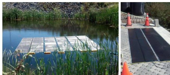
Figure 31: Thin film panels 570 W experimental floating plant (left) and the control array of 190 W (right), used by Trapani et al. [27].
