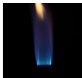
Figure 6: Flame observed in Tube 1 with flow rate 0.5 SLPM.
