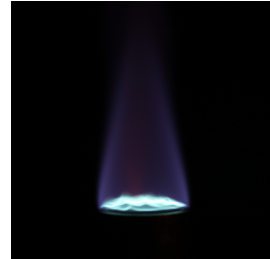
Figure 2: Flame observed in Tube 6 with flow rate 0.5 SLPM.
