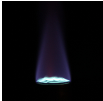
Figure 5.2: Flame observed in Tube 6 with gas flow rate of 0.5 SLPM.
