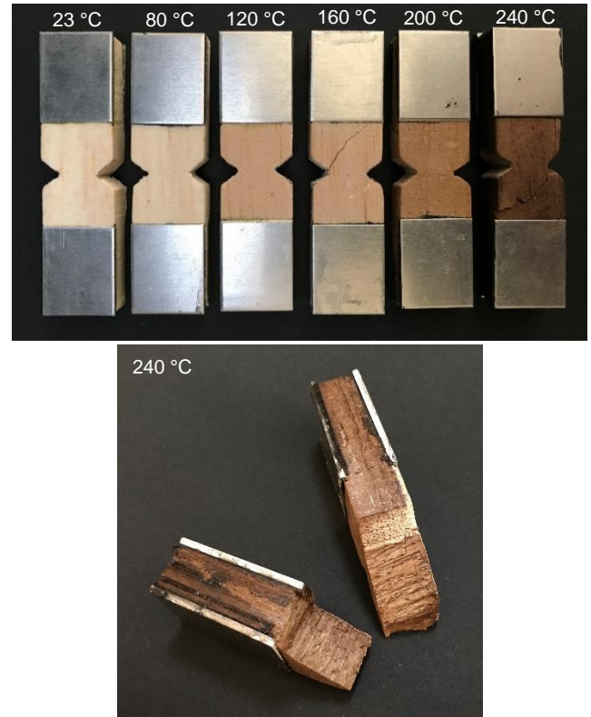
Figure 6 - Physical changes on the balsa wood with the temperature rise on the RT samples
