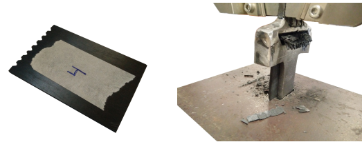
(a) Test specimens cut at 0° (b) Setup used for specimen with small indentations on crushing the top.
