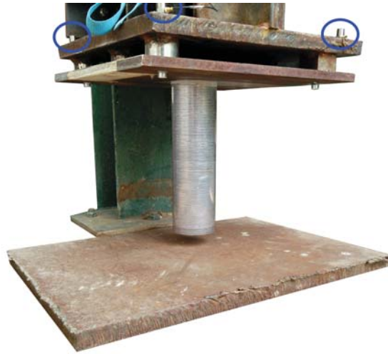
Figure 4.2: Aluminium tubes setup. The blue circles show the accelerometers position.
