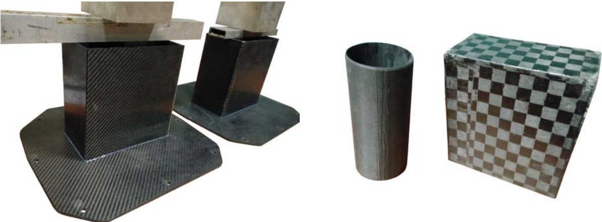
(a) Manufactured crashboxes while being glued to the AIP. (b) Alternative design ready to be glued to the AIP.
