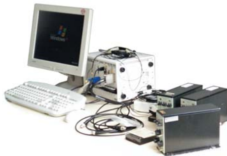
(a) Accelerometer data acquisition system.
