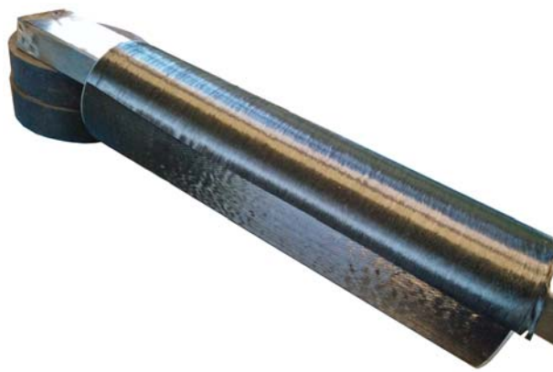
Figure 4.17: Manufactured carbon fibre tubes.
