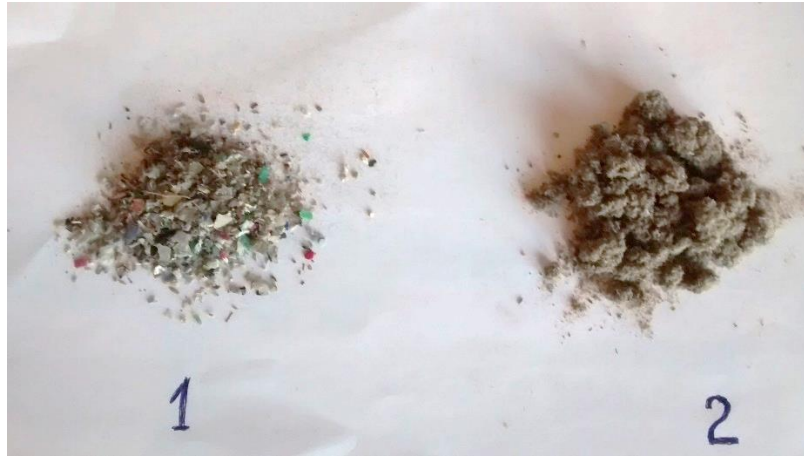
Figure 4 Studied RDF. 1 – original RDF, 2 – ground sample
