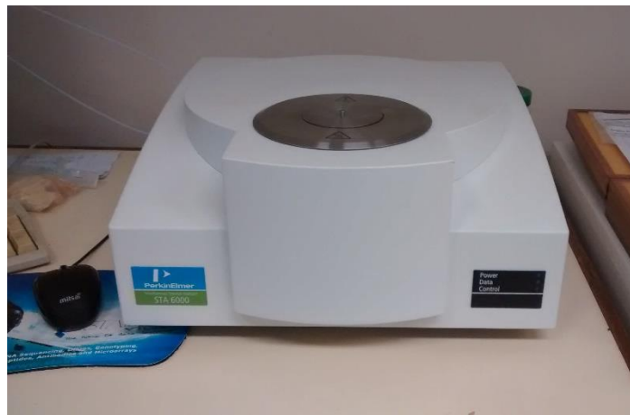
Figure 3 Simultaneous Thermal Analyzer (STA) 6000
