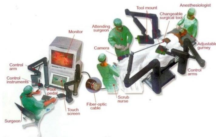
Figure 2 – Robotic system, that allows surgeons to operate at a distance.
