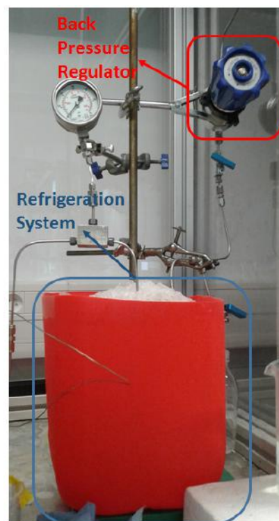
(c) Refrigeration system and Back pressure regulator.
