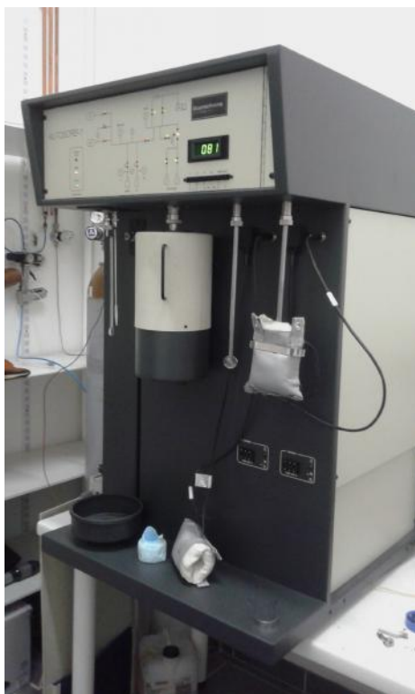
Figure 2.16: Illustration of a BET analysis equipment.
