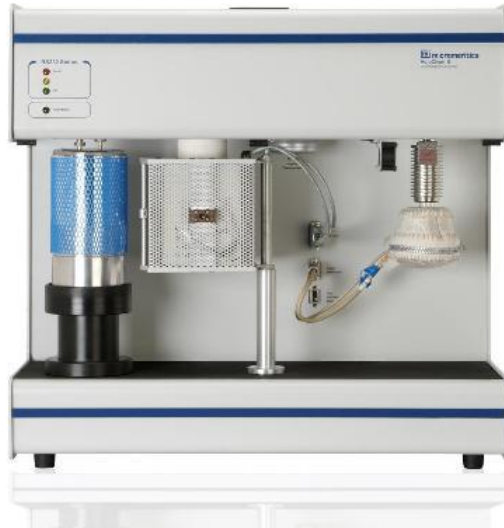
Figure 2.17: Illustration of a TPR analysis equipment. [76]
