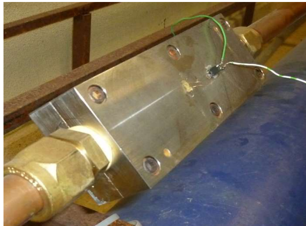
Figure 6.1. Assembled wall shear stress measurement structure
