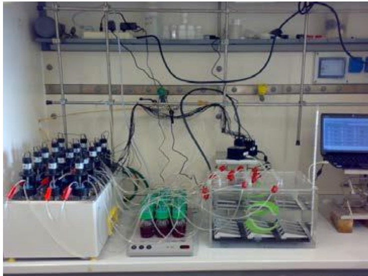
Figure 3.7 Example of BMP tests performed in the laboratory A.Rozzi, in the Cremona site of Politecnico di Milano
