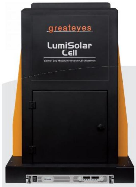
Figure 3.1: The luminescence setup at Solliance [3]
