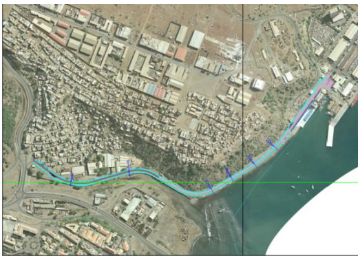
Figure 2.4: Extension of the road between Lém Ferreira and Port of Praia
