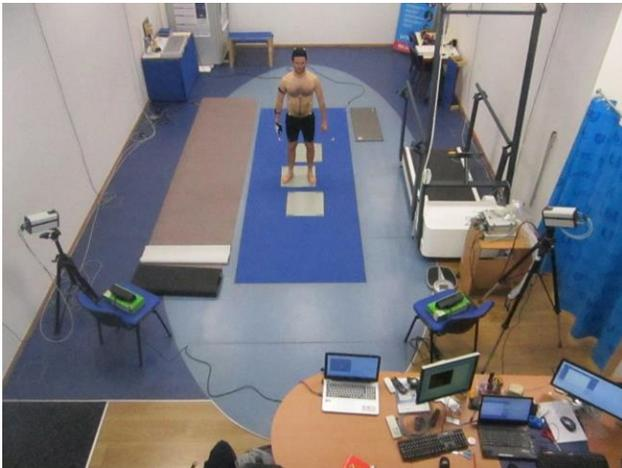
**Figure 9** - Photography of the workplace for the experiment. The subject is placed on the middle gray plate on the floor. Two Kinect sensors are placed, above a chair, on the right and left sides of the subject. Two of the fourteen IR cameras are also depicted on a tripod.
