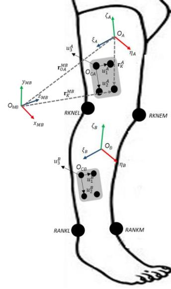
**Figure 11** - Representation of the local reference frames for the anatomical segments of the thigh, leg and clusters. The dash lines represent the position vectors regarding one tracking marker  $K$  of the thigh.
