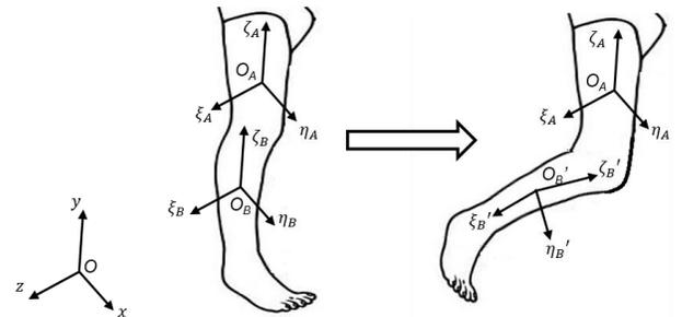
**Figure 2** - Representation of a knee flexion movement and its effect on the rigid bodies' reference frame. During the knee flexion movement, the leg's reference frame follows rotates around the  $\xi_B$ -axis leading to a new orientation. The thigh's reference frame remains static during the movement.
