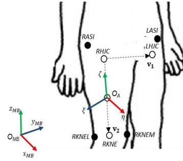
**Figure 5** - Local reference frame of the thigh on the marker-based system. The markers are illustrated by black dots while the points estimated from those by white dots.
