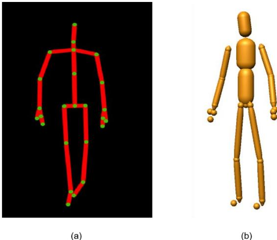
**Figure 1** - Skeleton tracked by the Kinect One sensor (a). Multibody system composed of 11 rigid bodies (b).
