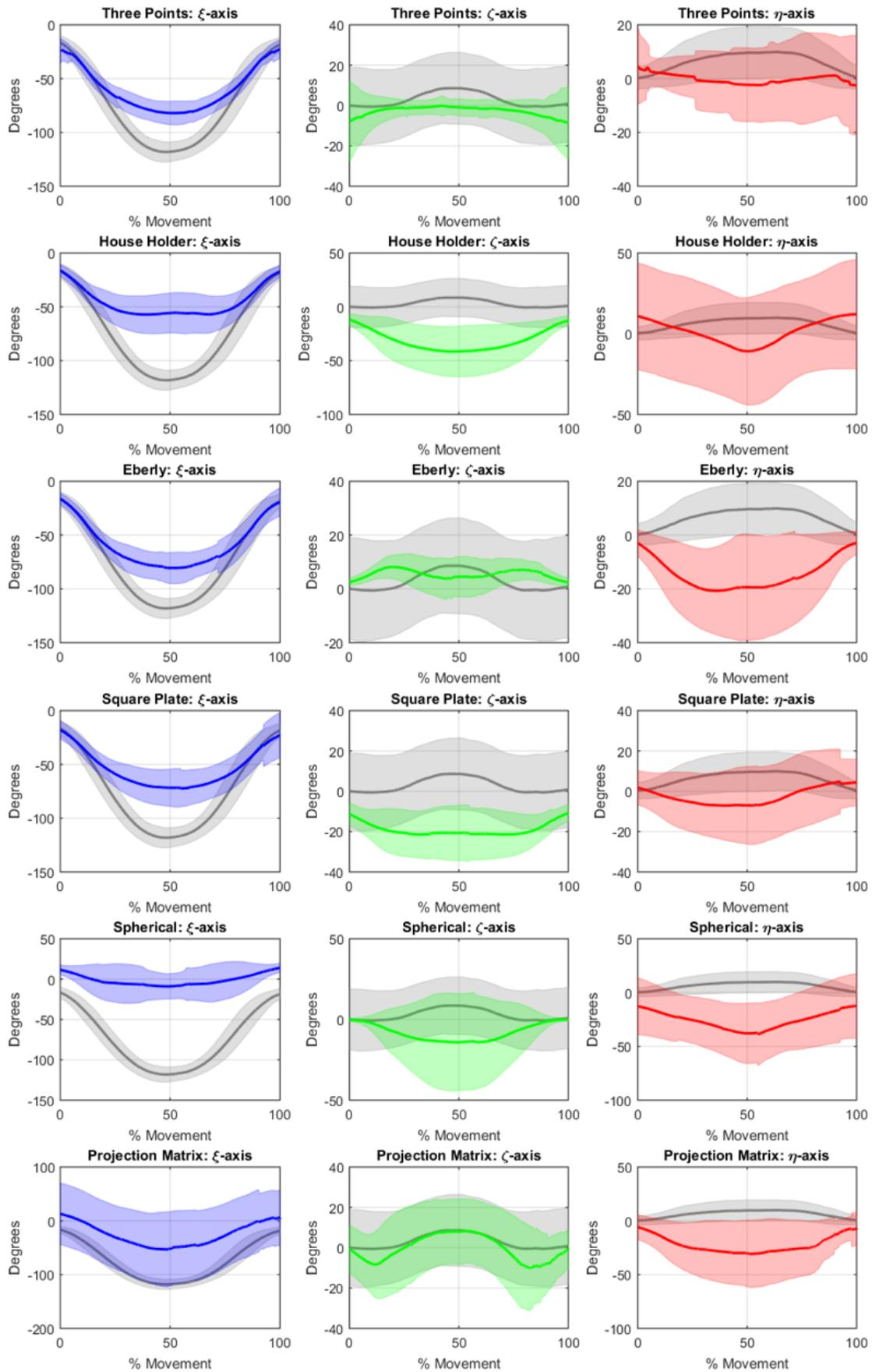
**Figure 13** - Orientation curves for the knee flexion movement for each technique applied on the marker-less system  $\pm 1SD$ . Each column represents the orientation around each axis of the reference frame. Each line represents one of the six techniques used (n=28).
