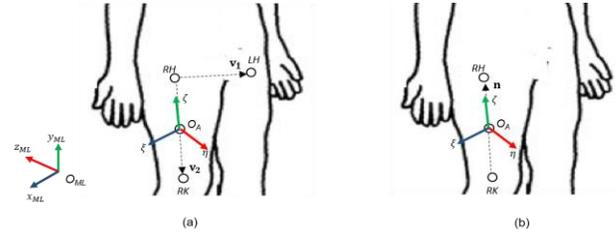
**Figure 6** - Local reference frame of the right thigh on the marker-less system. It can be reconstructed with three points by the TP technique (a) or with two points with one of the other techniques (b).
