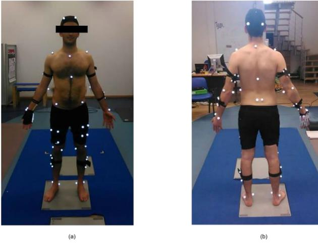
**Figure 3** - Photography of the marker-set with all the anatomical and tracking markers on the front (a) and on the back (b) for the marker-based motion capture system.
