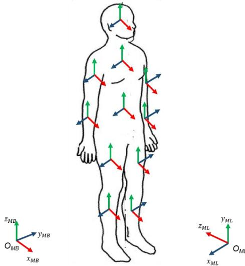
**Figure 4** - Representation of the full body with the local reference frames of each rigid body shown in the respective anatomical segments and the global reference frames depicted for each motion capture system.
