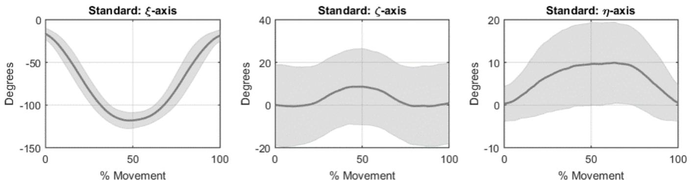
**Figure 12** - Orientation curves for the knee flexion movement on the marker-based system on the right leg segment. Each column represents the orientation around each axis of the reference frame  $\pm 1SD$  ( $n=28$ ).
