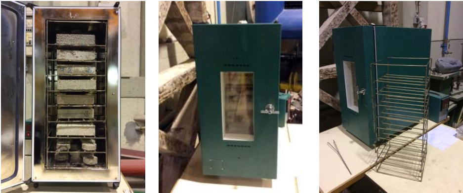
Figure 2 – Thermal chamber Tinius Olsen Environmental Chamber before and during the tests (left and center); metallic structure to hold samples during high temperatures exposure (right)
