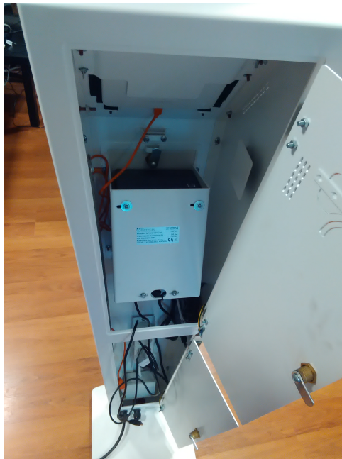
Figure 4.4: Photo of the kiosk from the back, with opened doors, where we see the tablet attached to the frame, the printer compartment.
