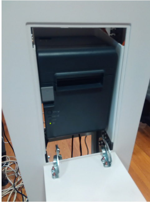
Figure 4.3: Photo of the kiosk with front door opened, detailing the printer fixed in its respective compartment.
