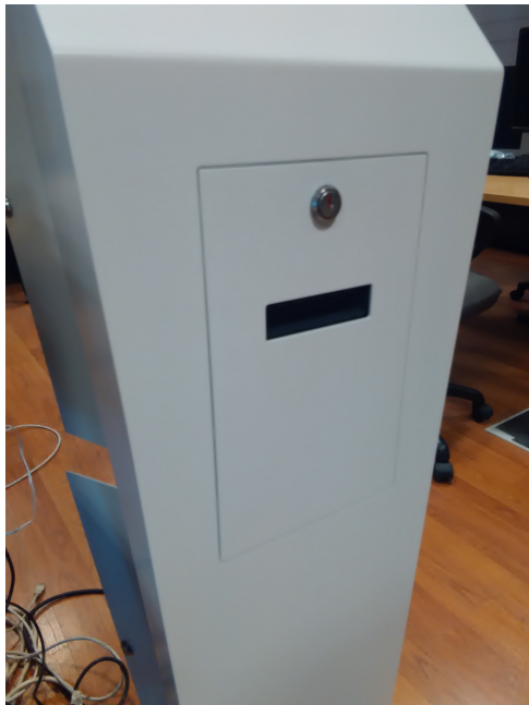
Figure 4.2: Photo of the kiosk detailing the slitted that aligns with printer and from where the ticket will come out.
