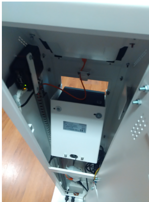
Figure 4.18: Picture of the kiosk from the back, with opened doors, where we see the tablet attached to the frame, the printer compartment, a left grey holder for the cable connections, power connection and plugs, and a hole in the bottom for other needed input cables, most notably needed for passing an Ethernet cable to the Raspberry Pi 3 used to control this system.
