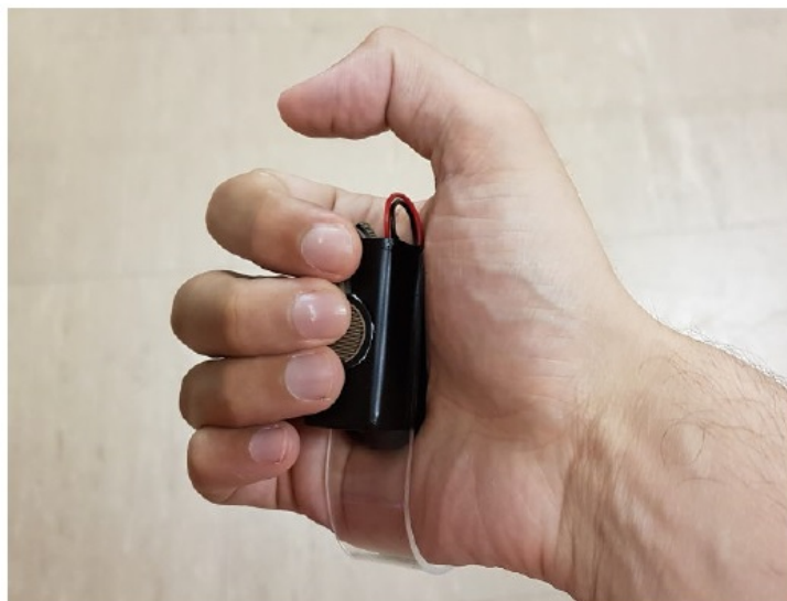
Figure 4.2: IMUduino. Our custom made device for hand tracking.
