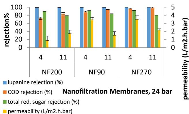
Figure 5 -Lupanine, COD and total reducing sugar rejections in the primary axis; permeability in the second axis for nanofiltration membranes at 24 bar.
