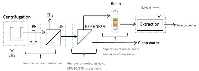
Figure 4 -Process diagram flow of a lupin bean wastewater treatment in industry. Starting from the left to the right: centrifugation, ultrafiltration, nanofiltration, resin and extraction operations are represented
