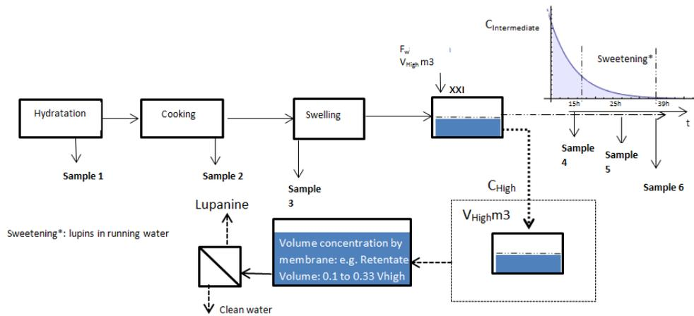
Figure 2 -Process scheme of one lupin bean industry A.
