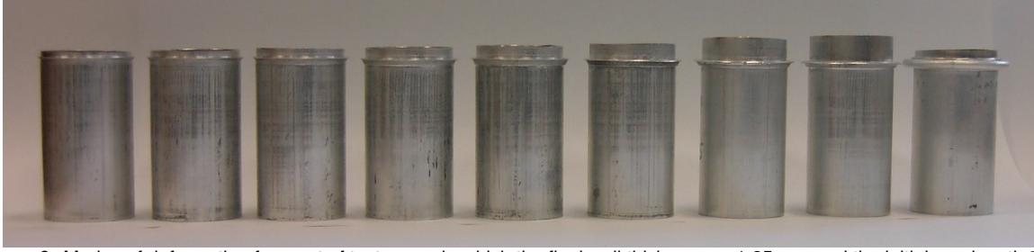
Figure 9: Modes of deformation for a set of test cases in which the final wall thickness t = 1.25 mm and the initial gap length l_{gap} varies from 5 to 16 mm (first row in Table 2).
