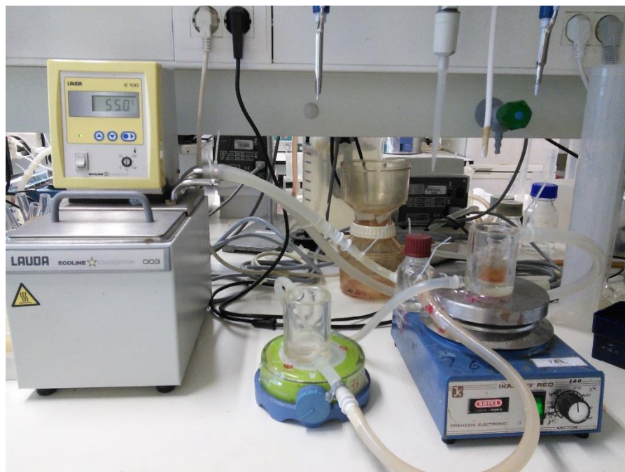
Figure 15 – General experimental setup for the biotransformation and enzyme activity measurements. In the picture Amberlite IRC-86 is being incubated inside jacketed vessel at 55°C in a reactional volume of 10 mL.
