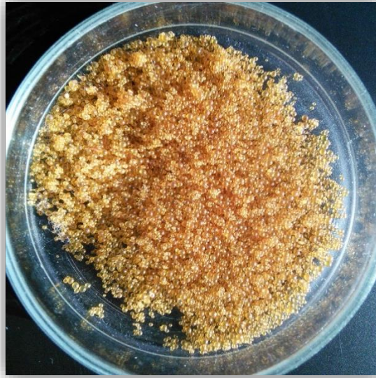
Figure 13 – Amberlite IRC-86 beads with a harmonic mean size of 0.58 to 0.78 mm. The functional group of this weak acid cation exchanger is carboxylic acid.
