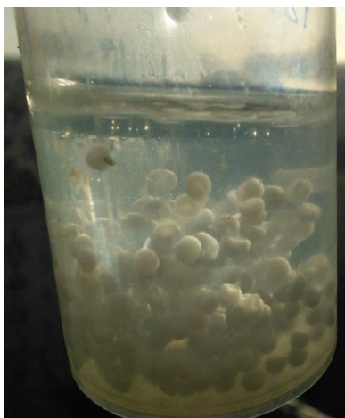
Figure 14 – Final form of the PVA beads in acetate buffer 0.1 M pH 4.5.
