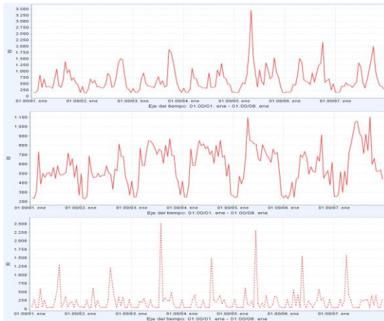
Figure 2 From top to bottom Polysun H45, G0 and H11 electricity consumption profiles for the first week of the year. (Polysun graphics).
