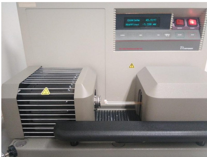
Figure 15 TA Instruments SDT 2960 Simultaneous DSC-TGA
