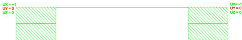
Figure 14: Applied boundary conditions in form of structural displacements in mm for a clamped-free-clamped-free plate in Ansys .
