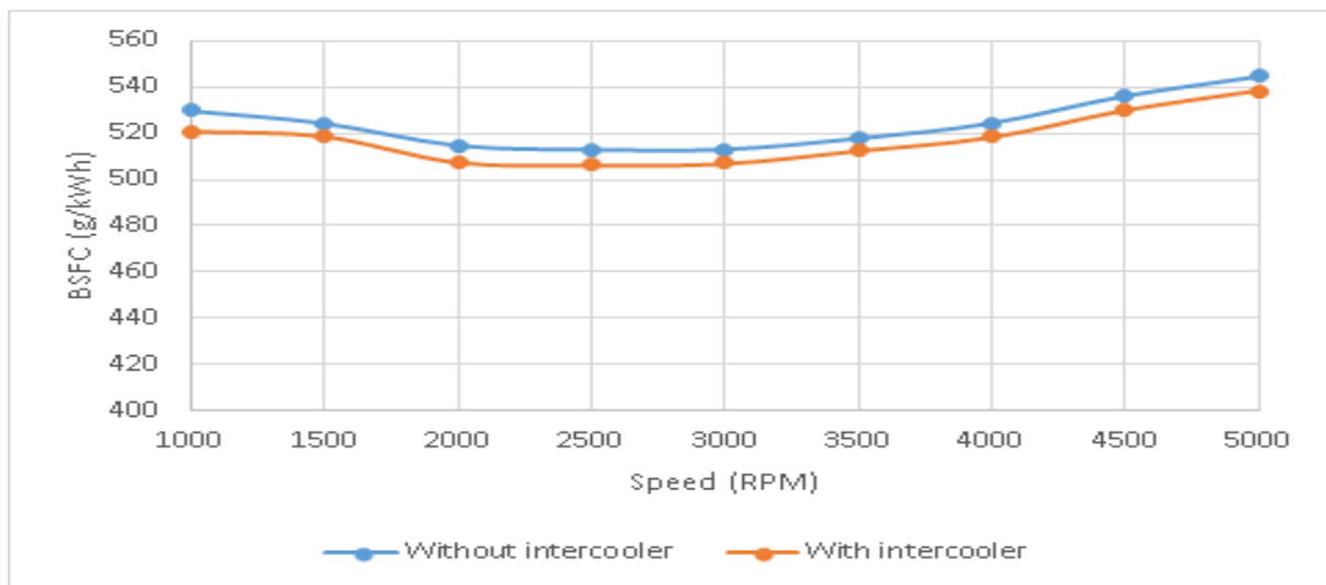
Figure 3.3: Comparison of BSFC between the cases with and without intercooler
