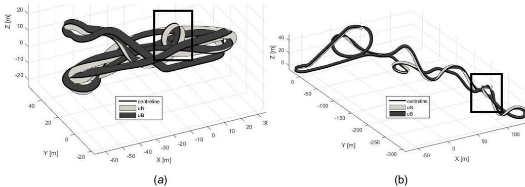
Figure 2.2: Three-dimensional representation of the track centreline and a sweep of the unitary normal and binormal vector. (a) Looping Star (b) Gate Keeper
