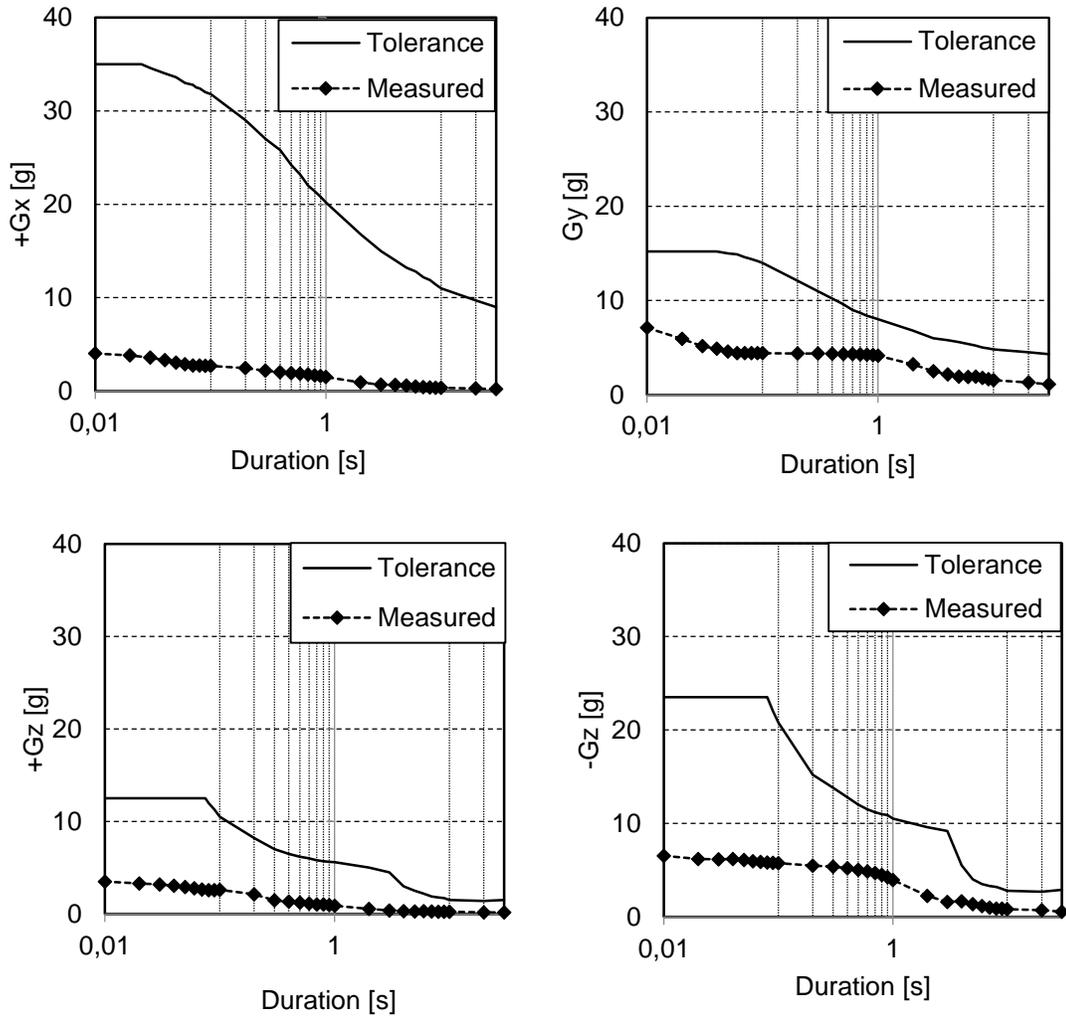
Figure 4.1: G-force acting on passenger for the Looping Star
