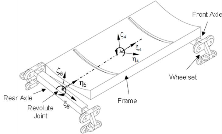
Figure 2.4: Primary Suspension System: Perspective
