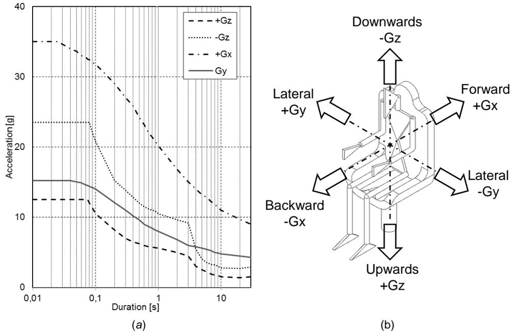
Figure 3.2: (a) Thresholds of human tolerance to g-forces, with respect to duration [4, 5]; (b) Nomenclature for acceleration components.
