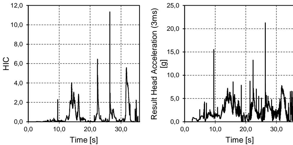
Figure 4.2: HIC and Result Head Acceleration (3ms) for the Looping Star
