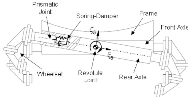
Figure 2.5: Primary Suspension System: Back View
