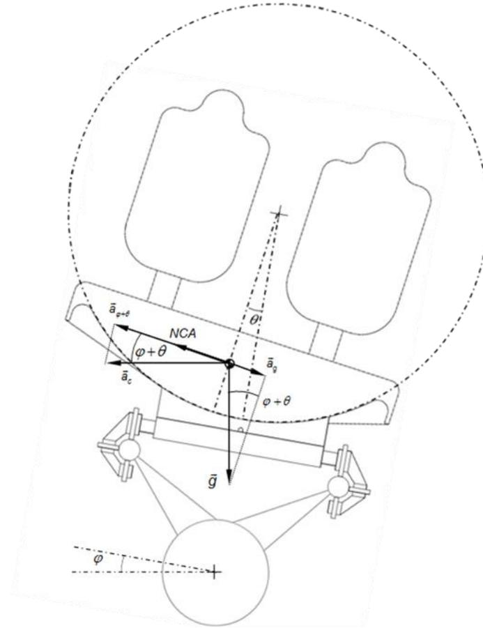
Figure 2.6: Graphical scheme to show the non-compensated acceleration (NCA)
