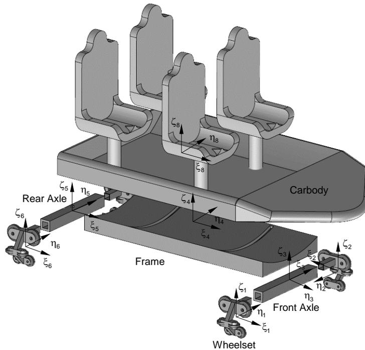
Figure 2.7: Geometric representation of body fixed frame for each individual body in the vehicle
