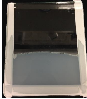
Figure 30 - Example of a hydrogel that became opaque after the polymerization reaction.
