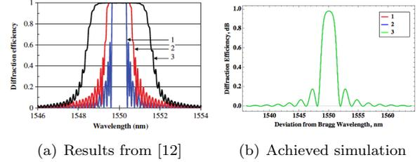
Figure 8: Modeled spectra of diffraction efficiency of CVBG with different spectral chirp rates (SCRs). Parameters of modeling: central wavelength  $\lambda_0 = 1550$  nm, spatial refractive index modulation  $\delta n = 700$  ppm, and thickness  $t = 5$  mm, SCR  $d\lambda/dz$ , nm/cm: 1-0; 2-0.5; and 3-5, respectively.
