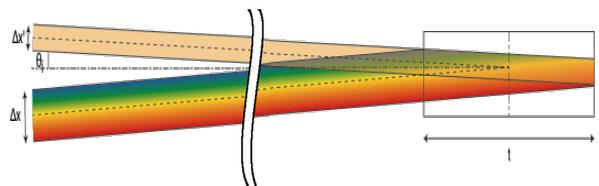
Figure 4: CVBG's top view depicting transversal chirp.
