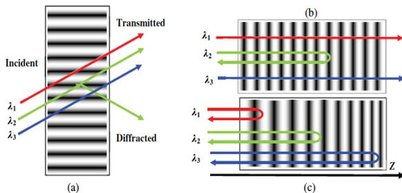
Figure 3: Schematics of beam diffraction by volume Bragg gratings. (a) Transmitting grating, (b) uniform reflecting grating (Bragg mirror), and (c) chirped reflecting grating,  $\lambda_1 > \lambda_2 > \lambda_3$ . Spatial modulation is not in scale: the typical period for a Bragg mirror at  $1 \mu\text{m}$  is about  $0.3 \mu\text{m}$  (from [12]).
