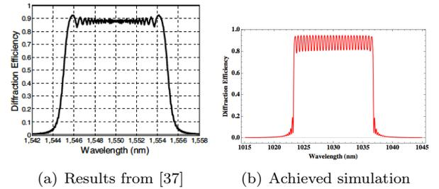
Figure 9: Diffraction efficiency of a CVBG, using partition methods. (a) grating parameters: Normal incidence,  $\lambda_0 = 1550$  nm,  $t = 10$  mm,  $N = 30$ ,  $n_{av} = 1.5$ ,  $\delta n = 800$  ppm; (b) grating parameters:  $\theta_i = 7.5^\circ$ ,  $\lambda_0 = 1030$  nm,  $t = 33$  mm,  $N = 30$ ,  $n_{av} = 1.499$ ,  $\delta n = 530$  ppm.
