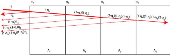
Figure 5: CVBG divided in 4 segments. The figure shows the amount of the initial beam that is diffracted by each of the individual reflecting gratings.
