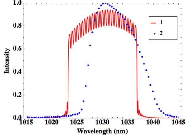
Figure 11: Comparison between experimental and simulated results. 1 - Diffraction efficiency of a CVBG, using partition methods. Grating parameters:  $\theta_i = 7.5^\circ$ ,  $\lambda_0 = 1030$  nm,  $t = 33$  mm,  $N = 30$ ,  $n_{av} = 1.499$ ,  $\delta n = 530$  ppm. (b); 2 - Reflected Beam at  $\theta_i = 7.5^\circ$
