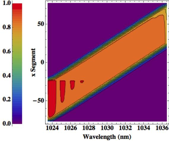
Figure 10: Spatial Chirp simulation, where hotter colours correspond higher intensities. Purple: 0 Intensity; Orange: Intensity = 0.9; Grating parameters:  $\theta_i = 7.5^\circ$ ,  $\lambda_0 = 1030$  nm,  $t = 33$  mm,  $N = 30$ ,  $n_{av} = 1.499$ ,  $\delta n = 530$  ppm.
