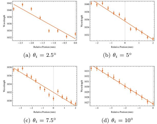
Figure 12: Horizontal chirp analysis for reflected beams, for several incident angles. Relation between central wavelength and its relative position in the beam.
