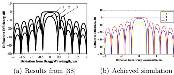
Figure 7: Dependence of diffraction efficiency of a RVBG on deviation from resonant wavelength  $\lambda_0 = 1985$  nm, for monochromatic plane waves at normal incidence. Thickness 1 mm, average refractive index  $n_{av} = 1.4867$ . Refractive index modulation, ppm: 1= 200, 2= 500, 3 =1000.
