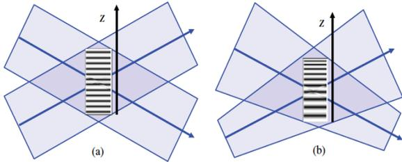
Figure 2: Recording geometry for uniform gratings by interference of collimated beams (a) and for chirped gratings by interference of a convergent and a divergent beams (b). Arrows show the direction of the recording beam propagation. Z is the axis collinear to the grating vector (from [12]).
