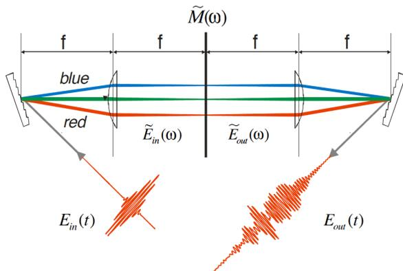
Figure 1: Basic layout for Fourier transform femtosecond pulse shaping (from [13]).
