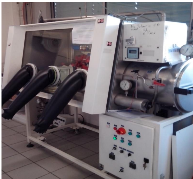
Figure 14- two-neck Schlenk (a) and Glove box (b) used during experiments
