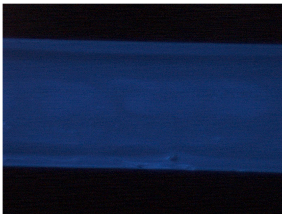
FIGURE 1.3: Microscopy photograph taken of a microfluidic channel patterned with a HRP labelled antibody. The photo was taken while running luminol through the channel at a 5 \mu\text{l min}^{-1} flow rate.
