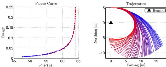
Figure II.2: Pareto curve and the trajectories corresponding to each optimal solution (in the same color) for the problem of minimizing the FIM determinant and the energy consumption by the vehicle.
