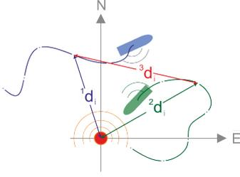
Figure II.4: Single-beacon navigation with two vehicles exchanging range information.
