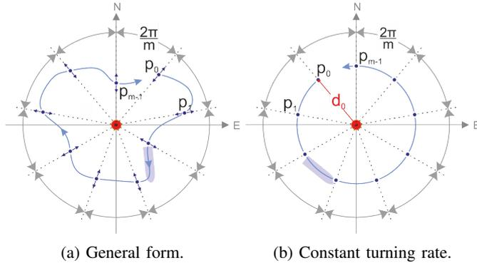
Figure II.1: Optimal trajectories for maximizing the FIM determinant imposing no limitations on the input functions.
