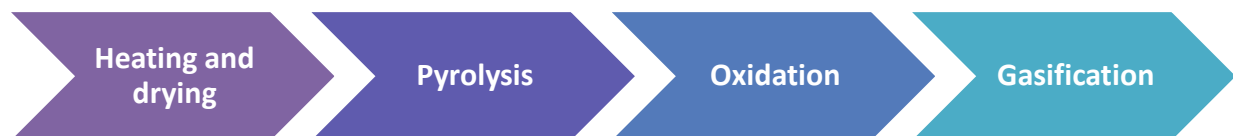
Figure 8 Gasification process steps (Source: Adapted from Ruiz, 2013)
