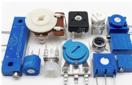
Figure 5.2: Potentiometers (or variable resistors, or rheostats) have a slider or a screw to move the position of a terminal, and thus the length of the resistor which is actually employed; resistance is proportional to this length, and can be varied in this manner (source: Wikimedia).
