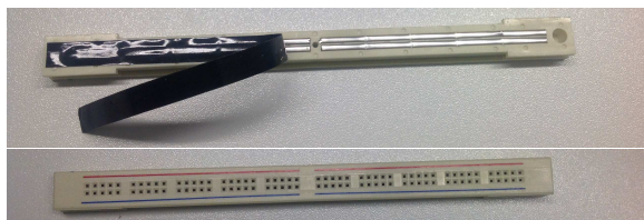
Figure 1.2: How breadboard perforations are connected.
