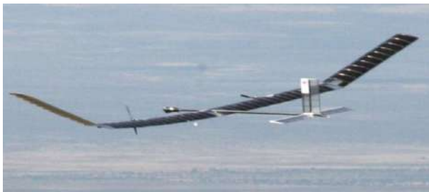
Figure 1: Airbus Zephyr HALE UAV
