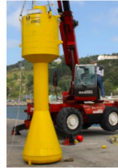
Figure 1. Oscillating Water Column 1/10 model of a spar-buoy device.
