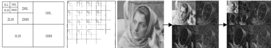
Figure 19 – DWT transformation on a single tile (left) [67], dyadic decomposition on the all set of tiles (middle) [63], example of the dyadic decomposition on the entire image (right) [67].
