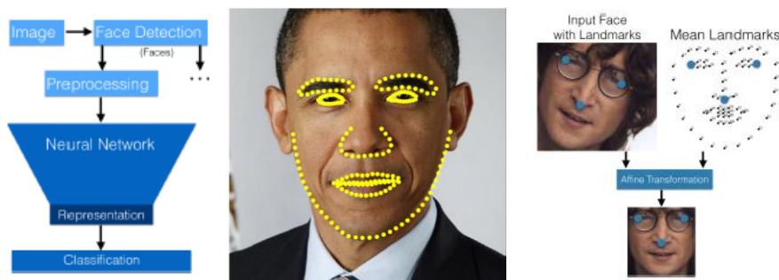
Figure 15 – Logic of face recognition systems that use NNs (left) [53], example of a 68 face landmark estimations on a real image (middle) [54], example of the affine transformation applied to a detected face in an image by using the blue points as reference (right) [53].
