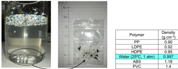
Figure 3: Separation of rPP(bulk) in a beaker and density data of the main polymers that could be present in the material.
