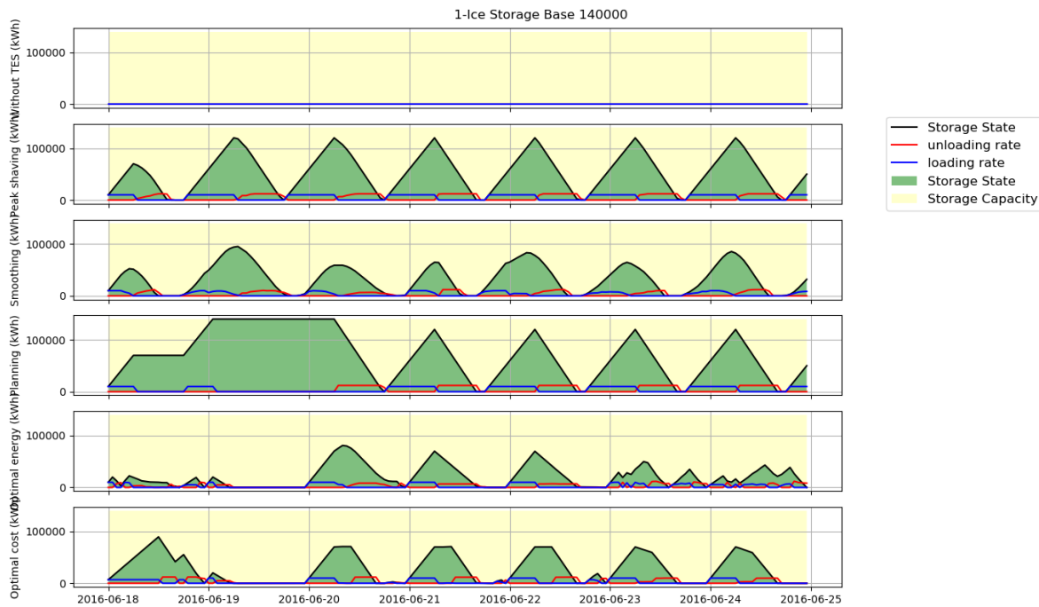
Figure 57 Storage state at different models for iced storage
