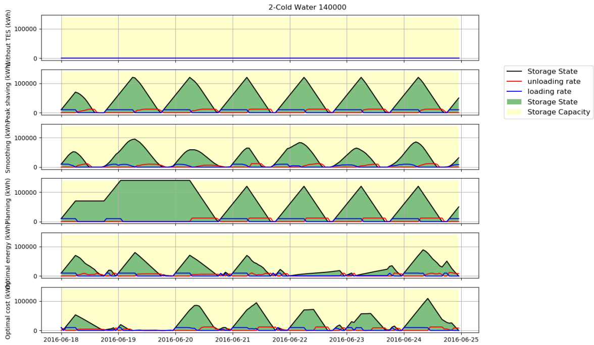
Figure 55 Storage state at different models for cold water storage
