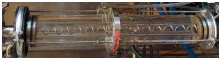
Figure 6. Oscillatory flow bioreactor jacketed module.
