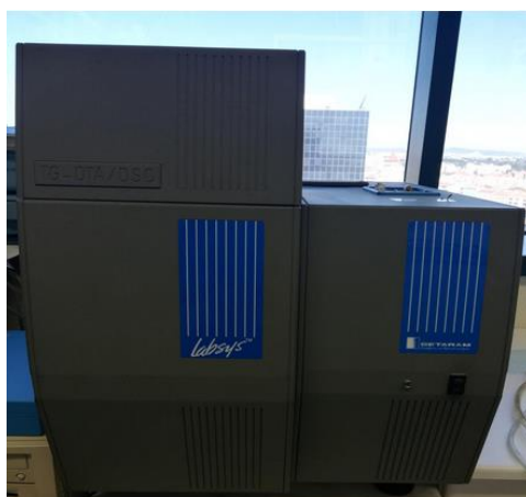
Figure 3-3 TG-DTA/DSC Sateram labsys
