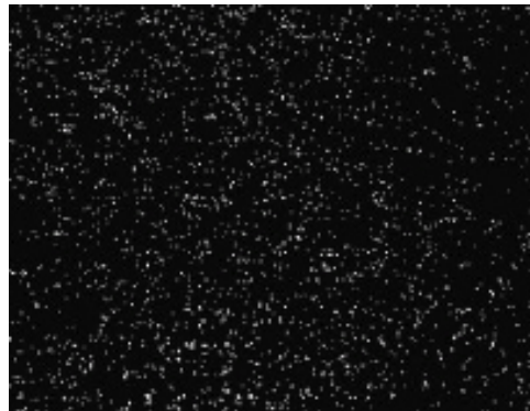
Figure 2.13: Appropriate particle density and illumination reference. Source: [56].
