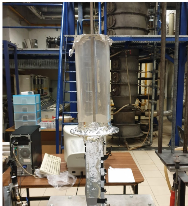
Figure 2.17: Experimental setup for the flue gas analysis: connection between the hood and burner.
