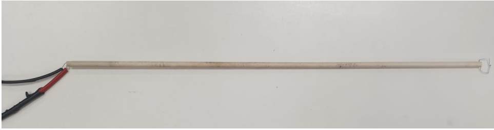
Figure 2.20: Thermocouple type R with a 65 \mu\text{m} diameter.
