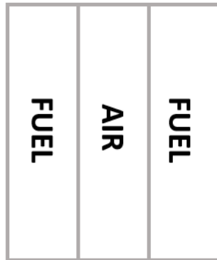
Figure 1.3: Schematic top view of the multi-slit rectangular burner.
