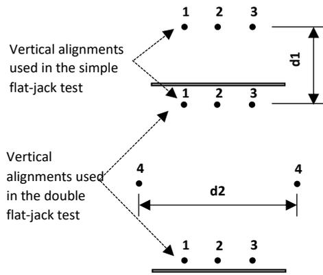
Figure 2 - Schematics of flat-jack tests
