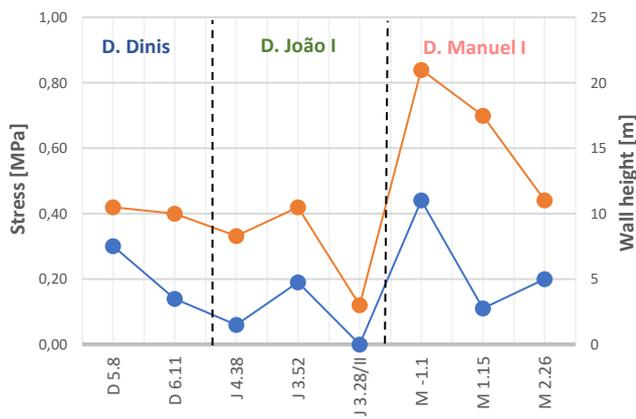
Figure 6 - Relation between in situ stress levels and wall height over the testing location
