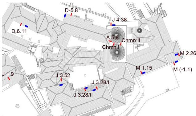
Figure 1 - Location of the studied masonries: red - core extraction; blue - masonry panels flat-jack and GPR tests
