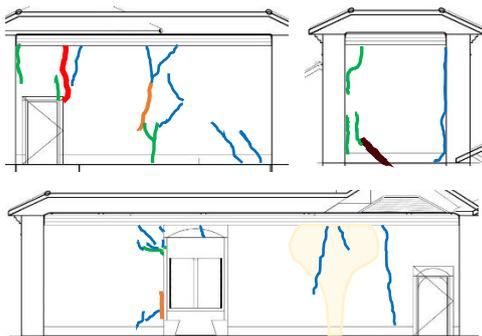
Figure 13 – Examples of the mapping of masonry wall anomalies (pale orange represents humidity stains
