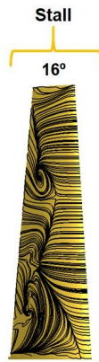
Figure 5.14: Streamlines of the flow in the upper surface of the wing for AoA: 16^\circ .
