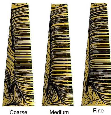
Figure 5.1: Limiting streamlines contours for the three different mesh densities: AoA=12 °.
