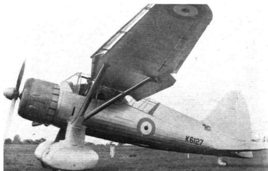
Figure 2.1: Handley Page Automatic Slot [11].
