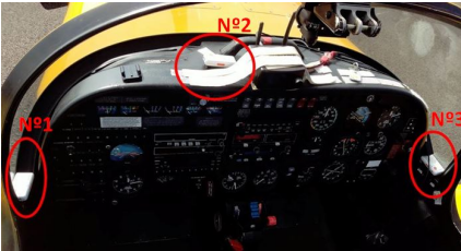
Figure 4.17: Sensor's position inside the cockpit.
