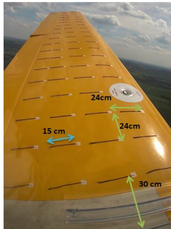
Figure 4.16: Wool tufts scheme on the upper surface of the wing.
