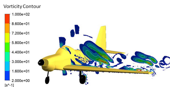
Figure 4.11: Vorticity Contour for the steady RANS flow calculations for an AoA = 18° .
