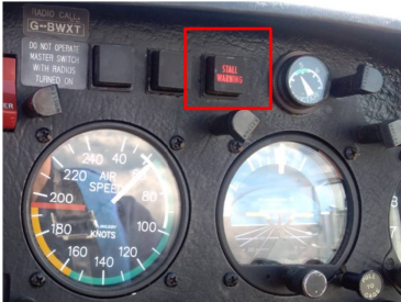
Figure 4.18: Stall warning of the Slingsby Firefly.
