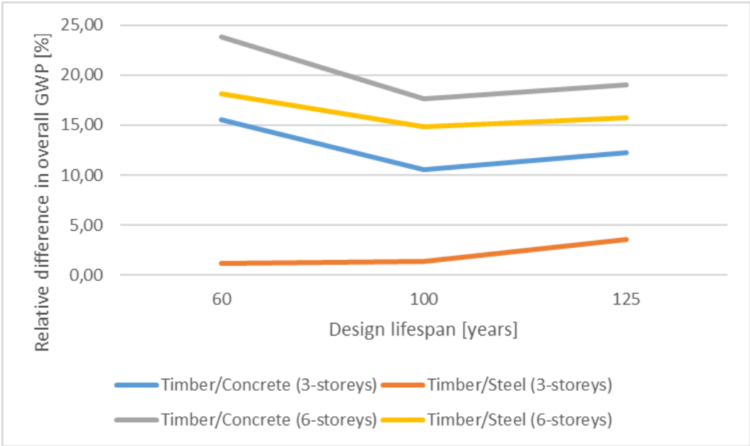
Figure 8.24: Relative difference in overall GWP when building with timber, ranged according to an increasing lifespan
