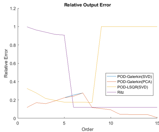
Figure 3.20: Relative output error evolution in relation to the ROMs's order.
