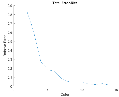
Figure 3.14: Total error of the solution corresponding to the static Ritz vector method
