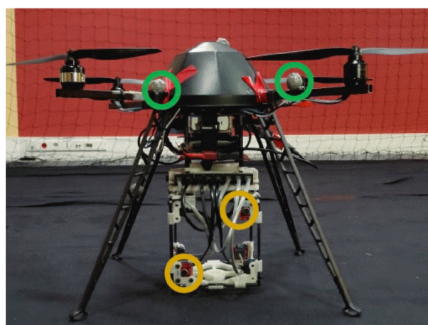
Figure 3.7: MikroKopter quadrotor with 8-channel microphone array.
