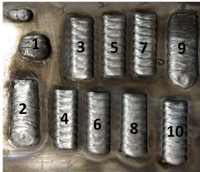
Figure 4.2: Experiments performed for the parametrization of the base of the final part
